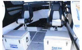
▲ A pair of Waeco Cool-Ice moveable chiller box seats that can be positioned anywhere in the cockpit.
